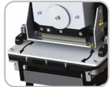
Belt Clamps on edge of support table **SECURE VARIOUS PROFILED BELT** in place.
