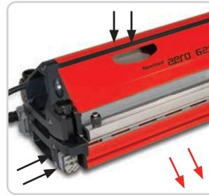
**Integrated Air Cooling** – cooling fans are positioned in both **top and bottom beams**, reducing cool down time after splice is complete. **Average splice times of 8-12 minutes** can be expected.
