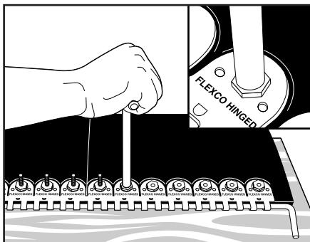
**13.** Break-off excess bolt ends using a Flexco Bolt Breaker. Use a slight rocking motion, parallel to the splice, while keeping the bolt breaker down tight on the nut.
