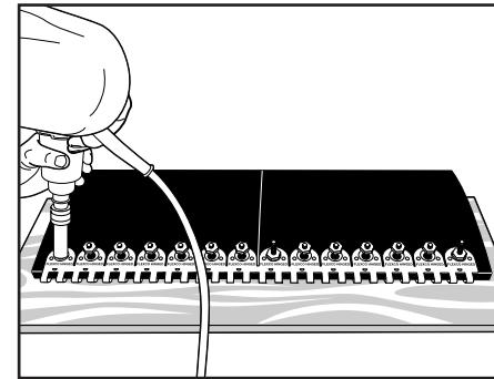
**9.** Using Flexco Power Wrench (H100) or Flexco Hand Wrench (100) tighten the nuts in the center and end plates.
