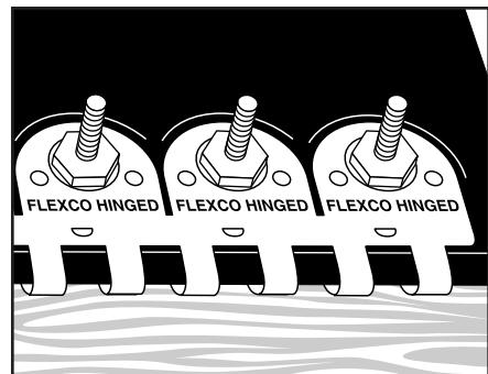
**11.** Fastener teeth should penetrate the bottom of the belt. Belt should pucker around the fastener edges.
