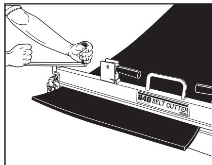
2b. For belt widths greater than 72" (1800 mm), use Flexco 840 Series Belt Cutter to make a straight cut across the belt.
