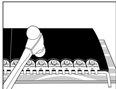
**14.** Peen or grind bolts to finish.
