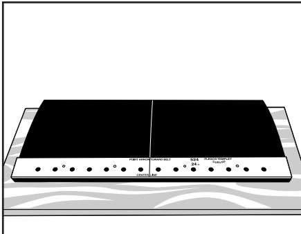
3. Place templet on belt, arrow on centerline. The arrow should point away from the belt end. Align templet edges with belt edges.
