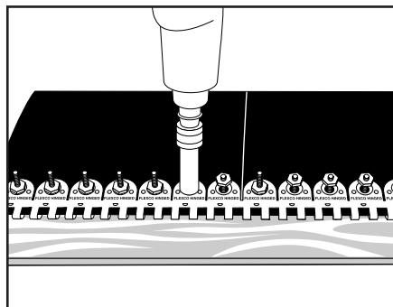
**10.** Tighten the remaining nuts from edges to center. Tighten uniformly. Trim excess Flexco-Lok® Tape.
