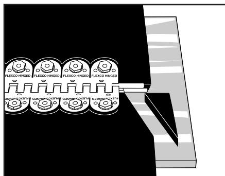
**18.** Notch trailing edges of belts 24" (600 mm) and wider.
