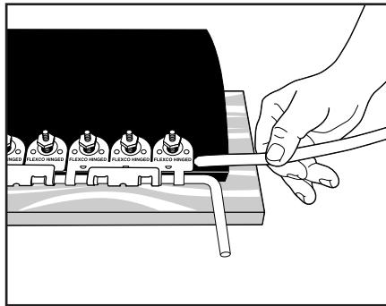
If Installing Individual Plates: Cut two strips of Flexco-Lok® Tape the width of the belt. Feed one strip under the top plates and one strip under the bottom plates.
