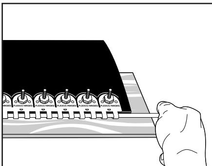
**12.** Insert gauge pin into fastener loops.
