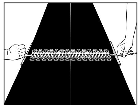
**17.** Insert gauge pin and feed the hinge pin from the opposite side of the splice while backing out the gauge pin.
