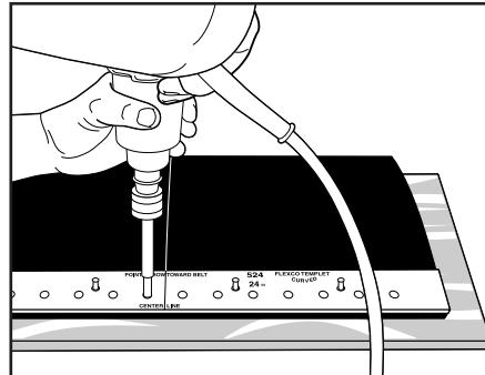
5. Punch bolt holes using either Power Punch (HP1) or Hand Punch (P1P). Use Power Wrench and impact tool for quicker installation. Max torque: 250 Lb-Ft (340 N-m).
