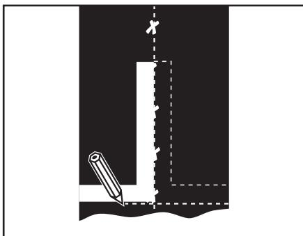
1. Square belt ends using centerline method.
