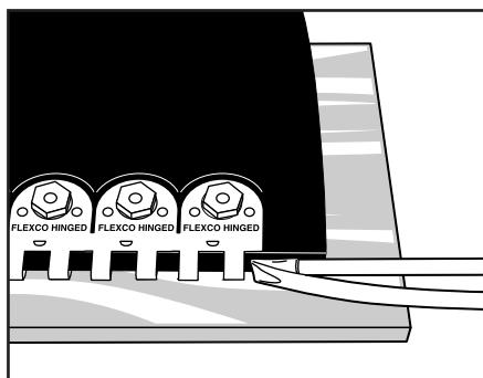
**15.** Insert filler tubing into the fastener loops. Use the gauge pin to guide the filler tubing into place. Pull out the gauge pin.
