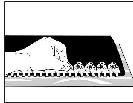
**8.** Assemble bolts and nuts. Turn nuts by hand until bolts engage lugs on fasteners.
