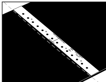
2a. For belt widths 72" (1800 mm) or less, use Alligator® 400 Series Curved Belt Cutter to make a concave cut across the belt.
