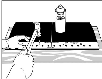
4. Nail templet to belt. Spray templet holes with Flexco® Silicone Lubricant.
