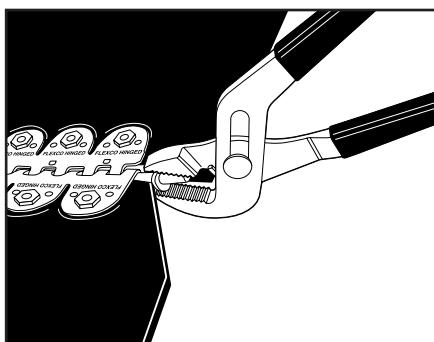
**19.** Insert washer on hinge pin and crimp with pliers.
