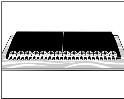
**7.** Place fastener strip on belt end with Flexco® Hinged facing up.
