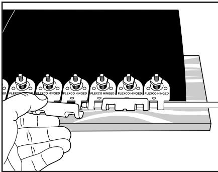
If Installing Individual Plates: Place a clip on the loops of the plates and insert gauge pin, repeat across the belt width.
