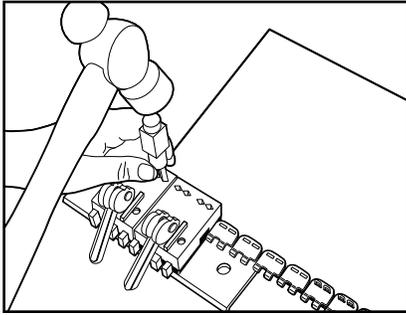
7. Drive belt ends next. Raise cam lever(s). Reposition tool, repeating step 5. Strike staple driver with a 1 lb. (0.5 kg) hammer.
