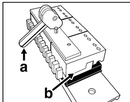
4. **Tighten** cam lever(s) until resistance is felt and back off 1/2 turn. Depress (a) cam lever(s). Combs should be (b) flush with guide blocks.
