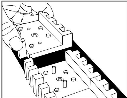
1. Insert the comb with the (a) fastener number that you are installing closest to where the fastener strip will be inserted.
