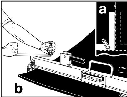
1. (a) Square belt using centerline method. (b) Cut belt using Alligator® 300 Series Wide Belt Cutter or Clipper® 845LD Belt Cutter.
