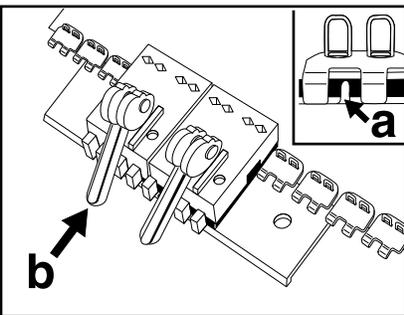
5. Belt end should be tight against the fastener (a) belt stops and fastener strip should be tight against the tool. (b) Depress cam lever(s).
