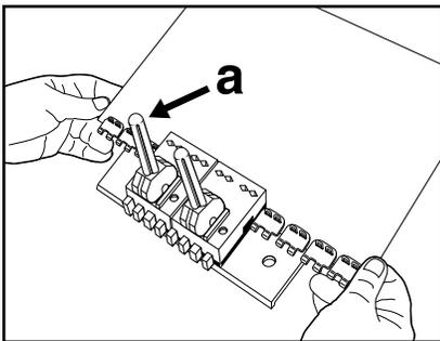
4. Center fastener strip in installation tool. (a) Cam lever(s) should be up.
