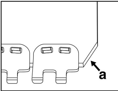
10. Using Belt Nippers, (a) notch trailing edge of belt only. Notch at an angle.
