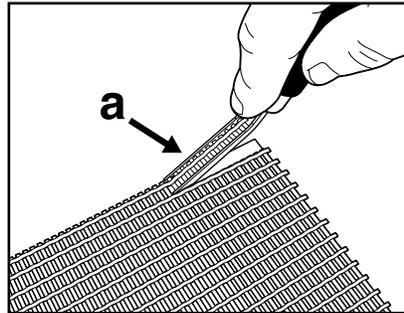
2. Select correct fastener size. See installation tool setup instructions. (a) Skive rough-top belt using Flexco skiving products.
