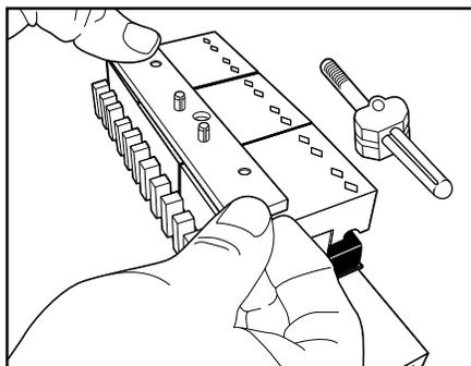
3. Replace clamp bar. Press down on clamp bar and/or guide blocks. Insert cam lever(s) and turn clockwise. Do not overtighten.
