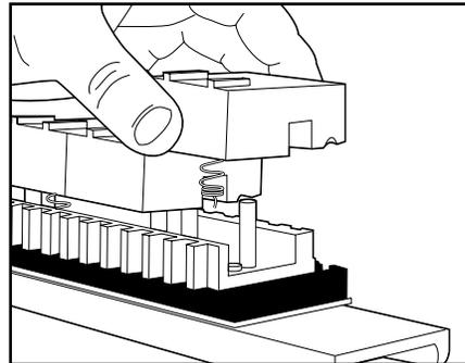
2. (a) Insert guide blocks. If using green guide blocks from C187, remove and replace with ST5-5 yellow guide blocks.
