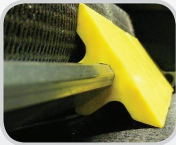
**Snap-fit design:** The 76 mm segments are designed to release under pressure if small objects become lodged between belt and segments.
