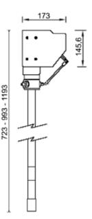
These pumps are suitable for the supply at high pressure of greases with viscosity up to NLGI 2 at short and long distances. The working pressure of the grease pumps here is 360 bar with a flow rate of 750 g/min.
